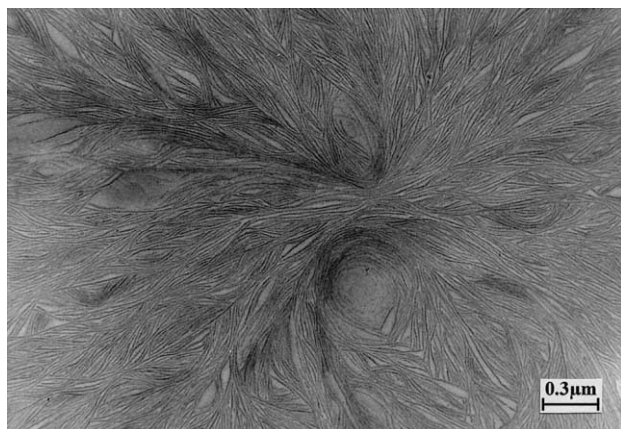
Fig. 7. BF electron micrograph of an iPS sample as in Fig. 6, which was further treated at 190°C (above the annealing peak, 175°C) for 1 min and then quenched to room temperature.
